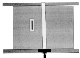
The fence is not parallel to the blade – it is skewed towards it at a slight angle.
