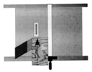
If you allow the stock to twist or skew, as soon as it reaches the back edge of the blade, the up-running teeth will launch it at you, in the direction of the blade rotation (red arrow).
